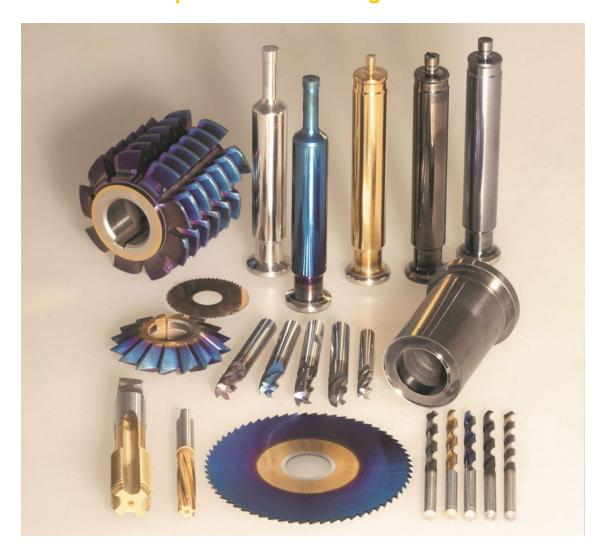
One of the industrially applicable technologies developed at the Jožef Stefan Insitute are hard protective coatings. On different coating machines deposition of various ceramic PVD hard coatings have been developed: TiN, CrN, TiAlN, AlTiN, TiAlSiN and aCN, as well
